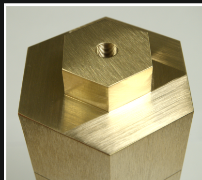
Brass hexagon piece, grained with absolute accuracy
