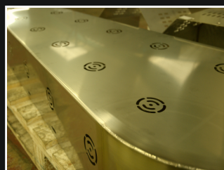
Stainless laser cut conveyor belt guard
